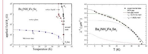
By synthesizing high quality  $Ba_x(NH_3)Fe_2Se_2$  superconductor we determined its superconducting phase diagram and its two-gap behavior of supercurrent density.
